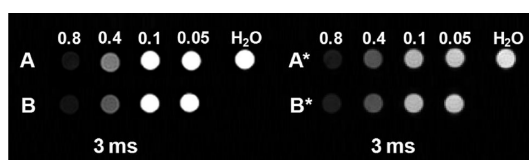
Figure 9. T_2 - and T_2^* -weighted images of radioluminescent nanocapsules. Group A: T_2 -weighted images of Gd 2 O 2 S:Eu nanocapsules with concentration of 0.8, 0.4, 0.1, and 0.05 mg/mL. Group B: T_2 -weighted images of Gd 2 O 2 S:Tb with concentration of 0.8, 0.4, 0.1, and 0.05 mg/mL. Group A*: T_2^* -weighted images of Gd 2 O 2 S:Eu nanocapsules with concentration of 0.8, 0.4, 0.1, and 0.05 mg/mL. Group B*: T_2^* -weighted images of Gd 2 O 2 S:Tb nanocapsules with concentration of 0.8, 0.4, 0.1, and 0.05 mg/mL.
